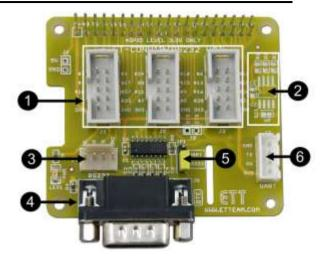
No.1 Connector IDC10 (J1, J2, J3) is arranged according to ETT Standard (PIN GPIOs of Board Raspberry Pi use 3.3V; it is not allowed to supply INPUT Voltage higher than 3.3V because the board maybe damaged).
