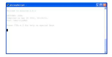
Type any text on Program minicom, user will see the text on the side of RS232 that is connected with computer as shown below; moreover, when type any text on the side of computer, user also see the text on the side of Raspberry Pi.
