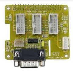
Board ET-CONV10/RS232 HAT is specifically designed for use with Board Raspberry Pi; it can be connected with INTERFACE Boards of ETT that use Connector as IDC10 type such as Board ET-OPTO RELAY4.
